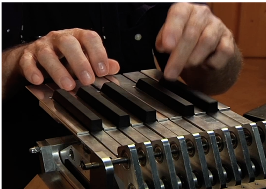
Fig. 1.7 Dispositivo aptico TGR (da JAMES LEONARD – CLAUDE CADOZ, Physical Modelling Concepts for a Collection of Multisensory Virtual Musical Instruments , in Proceedings of the International Conference on New Interfaces for Musical Expression , Baton Rouge 2015, p. 152).
