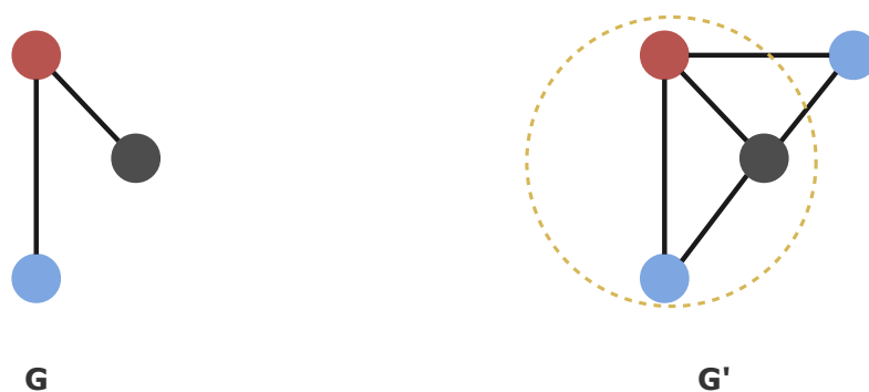
Figure 2.2: Graph G is a subgraph isomorphic to G' , the subgraph is highlighted in yellow. This is not induced, because in the subgraph of G' there is an extra edge.
