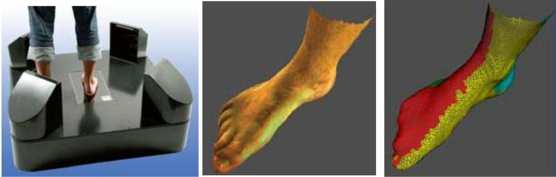
Figure II-28 Precision 3D Foot Scanner (Hometrica s.d.) (FotoScan 3D s.d.)
