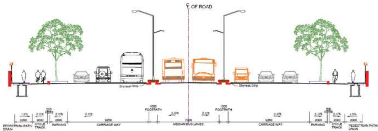
TYPICAL CROSS SECTION AT BUS STOP LOCATION 40M ROW
